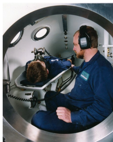
FIGURE 9: An inside view of the two-place mobile Cowan Manufacturing Company Transportable Recompression Chamber to be used in our prototype HBO 2 acute stroke treatment ambulance. Pure oxygen will be delivered to the patient via mask or hood, and the chamber itself will be pressurized with air at 2.5 ATA.
