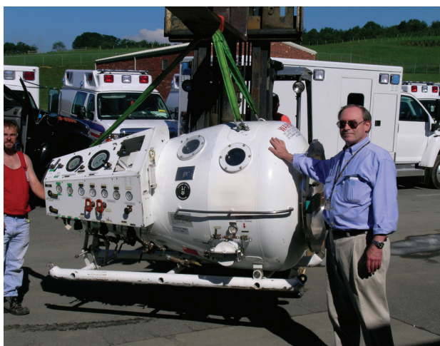
FIGURE 8: For the construction of our prototype HBO 2 chamber-equipped Acute Stroke Ambulance, we are using the two-place mobile Cowan Manufacturing Company Transportable Recompression Chamber.
