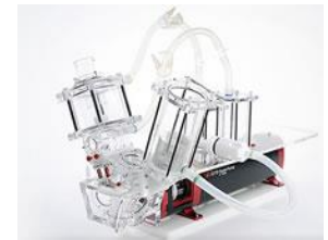
Pulse Duplicator for Hemodynamic Testing of Heart Valves
